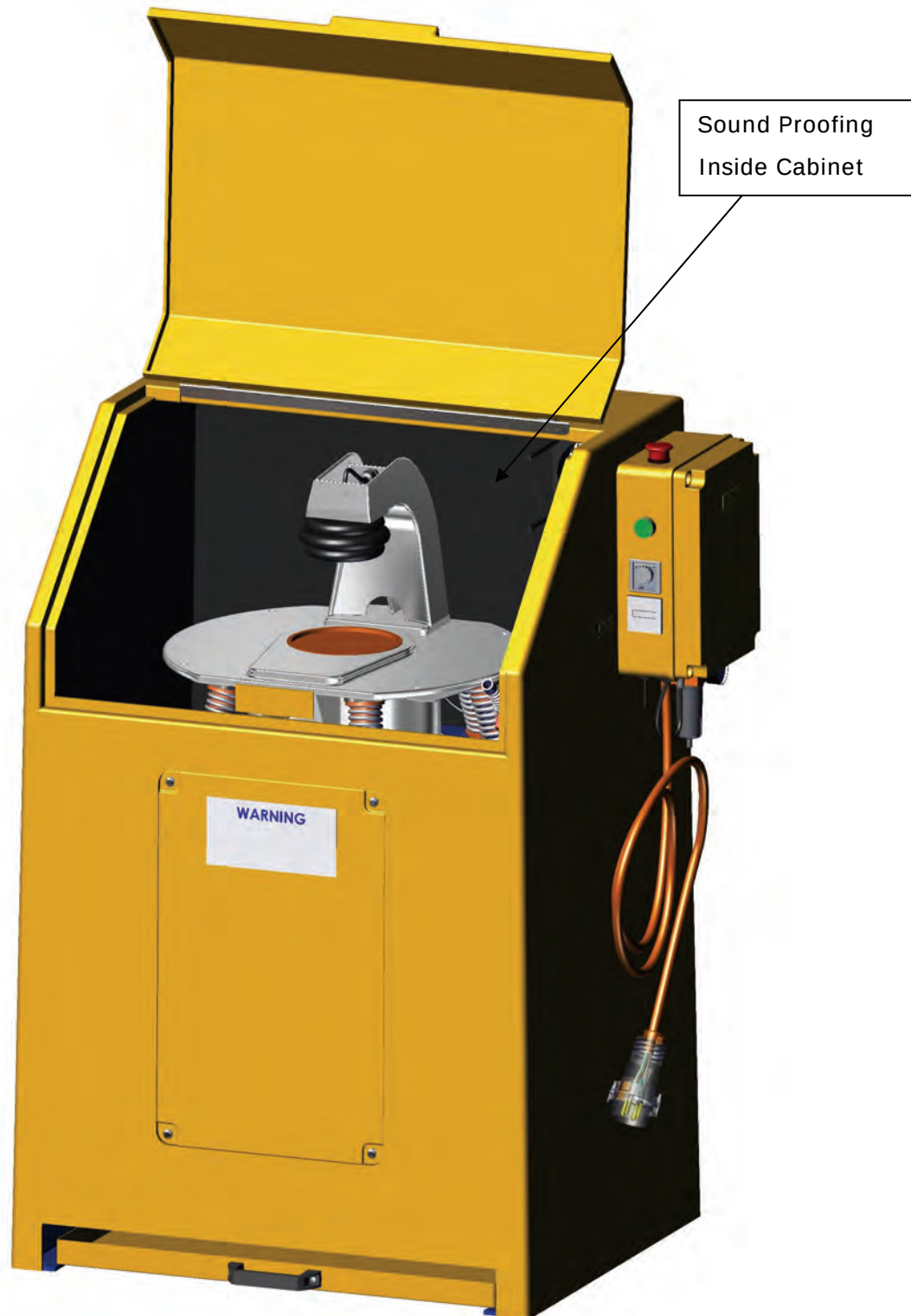
Figure 21 Replacement of Sound Proofing
