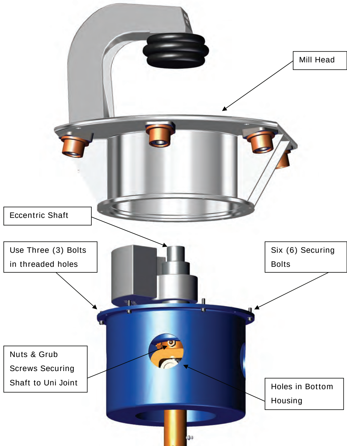
Figure 33 Separating the Mill Head from the Bottom Housing
