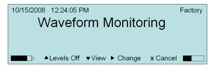
Highlight the Record Mode menu option and press the Right Arrow key to access the menu. Continue to press the Right Arrow key until the Waveform Record Mode option appears.
