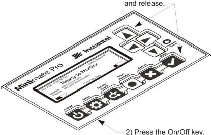
**NOTE:** A **Charging Status** LED is located next to the **Down Arrow** key and indicates the following:
