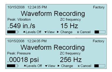
11. Press the **Cancel** key to stop recording, and the screen will return to **Main Display**. At any time, during, before or after, you can push the **Down Arrow** key to turn **Levels Off** and the display will no longer be updated with the **Peak** and **ZC Frequency** information.
