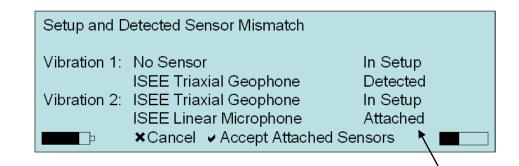
THIS COLUMN INDICATES MISMATCHED SENSORS. FOR EACH CHANNEL THE SENSOR THAT IS IN THE SETUP IS LISTED, AND THEN WHAT IS ACTUALLY ATTACHED TO THE UNIT.
