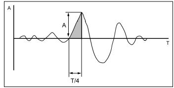
Manual Waveform Calculations on Nearly Triangular Waveforms
