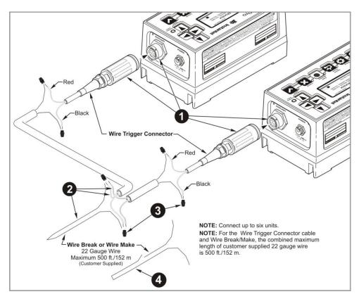
Multiple Wire Break/Make Trigger Cable Setup
