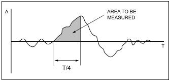
Manual Waveform Calculations on Irregular Waveforms
