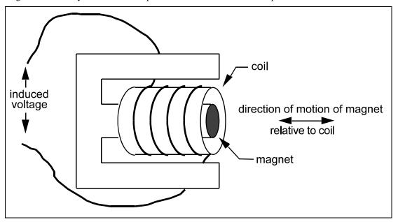
Figure 10.1 Geophone Sensor Operation.
