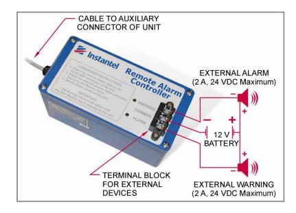
The Remote Alarm Controller indicates normal and over-triggering at a remote site. Use an optional extension cable to extend the length of the input cable; the output from the terminal block of the Remote Alarm Controller box can be used to run long distances to drive an external alarm.
