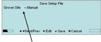
Use the **Right** and **Left Arrow** to navigate the text field, and the **Up** or **Down Arrow** to **Change** the characters
