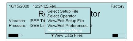
2. Press the **Up** or **Down Arrow** keys on the unit to highlight Next/Prev Setup Maintenance Menu options. Press the **Right Arrow** key to Action a Maintenance Menu option. At any time, press the **Cancel** key to return to the previous screen.
