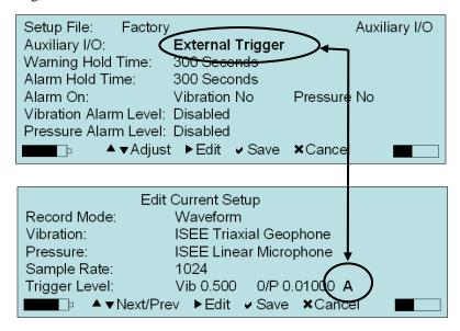
Follow the directions below to set the **Alarm Levels** within the **Auxiliary I/O** menu:
