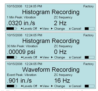
6. If a **Waveform** recording is triggered, then the information for **Pressure** and **Vibration** is also available while the **Waveform Recording** message is displayed:
