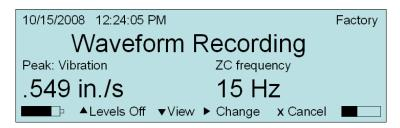
4. Press the **Right Arrow** to **Change** between **Peak Vibration** (shown above) and **Peak Overpressure** results. Below is an example of the **Peak: Pressure** and **ZC Frequency** readouts that are dynamically displayed:
