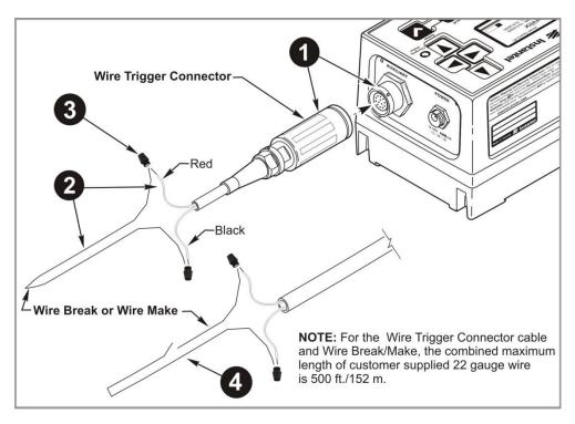
Single Wire Break/Make Trigger Cable Setup
