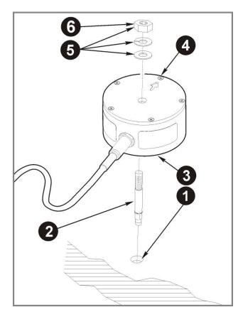
**NOTE:** If the Geophone is being mounted to the ceiling, the directional arrow must be mounted against the ceiling's surface to ensure that the orientation of the internal vertical transducer is correctly positioned. If it is not correctly positioned, the **Sensor Check** feature of the unit will indicate that the position of the Geophone needs to be checked.
