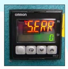
It could be a few things, the most common is the thermocouple is broken and needs changing.
