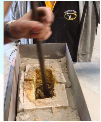
This Flue was "cleaned" but the operator failed to check down the flue with a flash.
