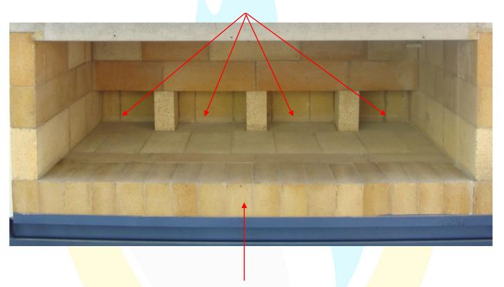
Knock off any Build up/spills that are on the front bricks.
