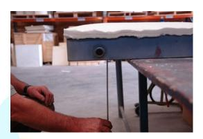
Place a screwdriver through the hole (kaowool side up) then the cutter over the screwdriver (a piece of pipe with a circumference of about 25mm by 100mm long with a mark about 50mm up). Keeping the cutter at 90 deg, cut down to marked line in cutter (50mm) and pull out. Knock out kaowool stuck in cutter.
