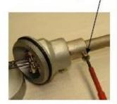
Make sure the screws in thermocouple head are tight, and are in correct position.
