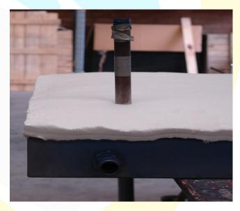
Once cutter is pulled out there is a hole big enough to place anchor through.
