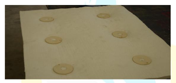
7. Once all anchors have been installed, use a straight edged, flat piece of wood and a sharp knife to cut off overhanging kaowool. Make sure the straight edge is lined up flush with the outer lip of furnace door top and bottom. Push straight edge down firmly and cut off excess kaowool.
